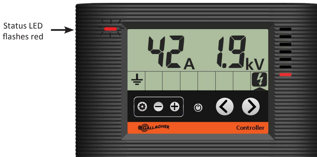
Controller showing the energizer in output alarm
